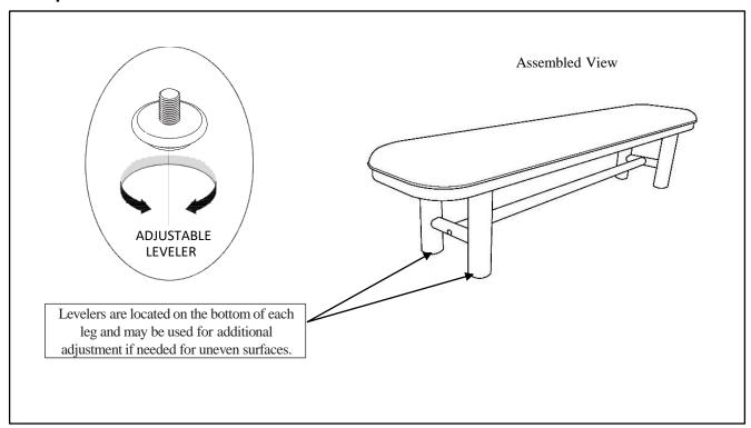
Assembly is now complete and the product is ready for use. Adjustable levelers are located on the bottom of each leg and may be adjusted by turning outwards, counter-clockwise to help account for uneven surfaces.
