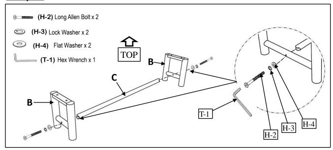
Position one Bench Leg (B) assembly with the end of the Stretcher (C), which should slightly wrap around the Bench Leg (B). Align the holes and secure connection with a Long Allen Bolt (H-2), Lock Washer (H-3) and Flat Washer (H-4) using the provided Hex Wrench (T-1), Stacking the hardware in the order as shown. Repeat the same process for the other Bench Leg (B) and the other end of the Stretcher (C). DO NOT YET FULLY TIGHTEN.
