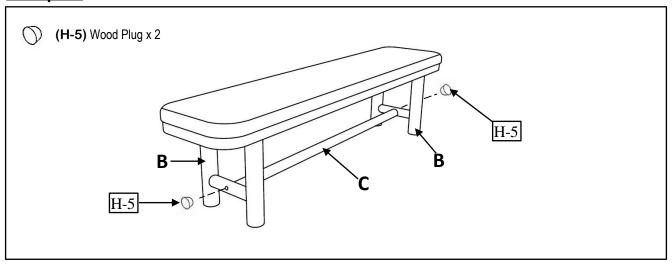
Using a second person to assist you, turn assembly uptight. Position the provided Wood Plugs (H-5) on each end. insert into the counter sink holes and firmly push by hand. DO NOT USE A MALLET, HAMMER, OR ANY OTHER TOOL.
