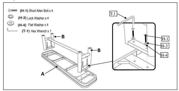
Using a second person to assist you, carefully lay the Bench Top (A) upside down on a padded, non-marring surface. Position the assembly from Step 1 onto the bottom of the Bench Top (A) and align the holes. Secure with Short Allen Bolts (H-1), Lock Washers (H-3) and Flat Washers (H-4) using the provided Hex Wrench (T-1), stacking the hardware in the order as shown. Fully tighten all hardware from this and the previous step. DO NOT OVER TIGHTEN.
